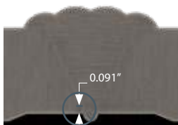
Flaw 3: Root Crack Length: 0.306"
