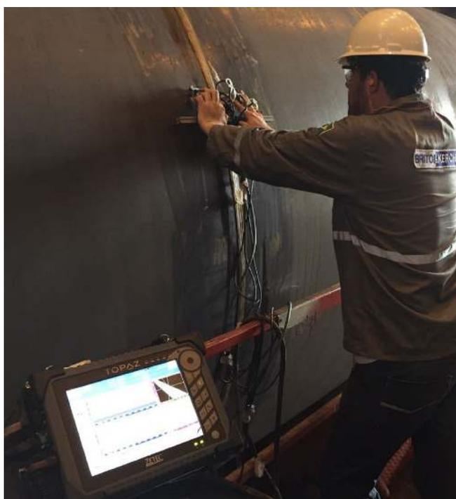
**Figure 1. The simultaneous use of phased array UT and TOFD can detect all welding flaw types and provide reliable through-wall sizing in one single inspection. They can produce higher detection capability, more accurate characterisations of corrosion and complete coverage of the material under test.**
