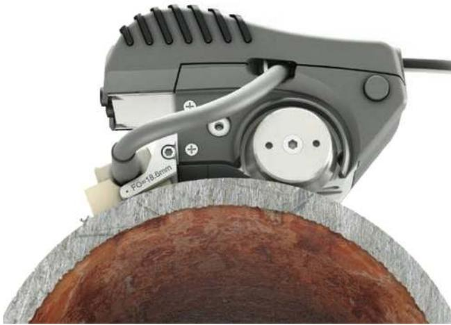
**Figure 3. A 2D encoded scanner like Zetec's NDT PaintBrush combines precise data collection with accurate positioning in any direction on flat or curved surfaces, ideal for mapping pipeline corrosion.**
